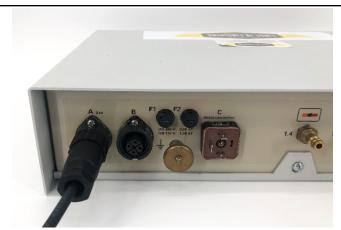
2. Attach Grounding Cable Assembly behind Grounding Nut
