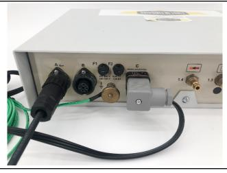
4. Attach Rinsing Air Assembly into 1.4 Fitting
