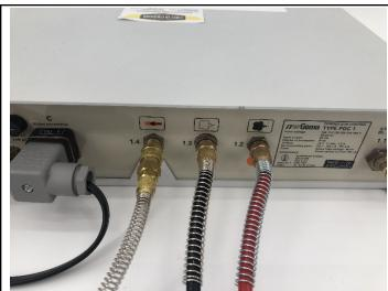
8. Attach other ends of Supplemental & Conveying Air to Powder Pump
