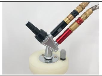
12. Attach Powder Hose Securely to Powder Hose Pump Connector
