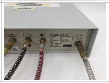
10. Attach Regulator End of Fluidization Assembly to Quick Disconnect On Powder Hopper
