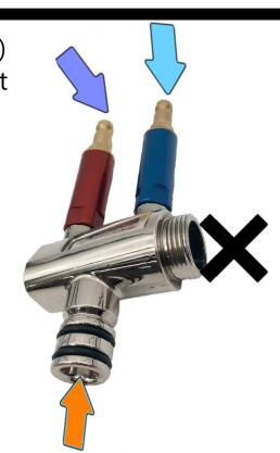
7. Blow Out Interior & Exterior of Pump Insert
